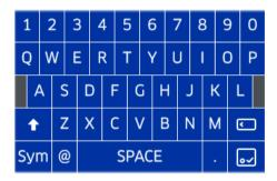
Note: Change case or symbols in the same way you would on your mobile telephone i.e. press the 'shift button' and the terminal will change to lower case characters or press the 'Sym' button and the terminal will display the special characters.
